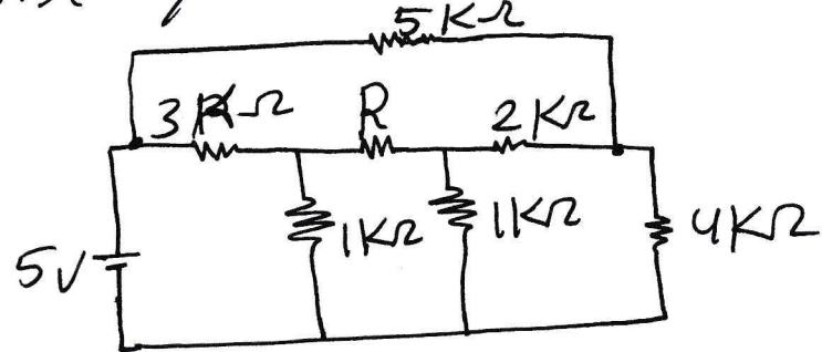
Q2/ Find  $I_1$ ,  $I_2$ , and  $I_3$  for Figure below.
