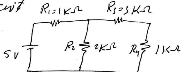
$$5 = R_1 I_1 + R_2 I_1 - R_2 I_2 \quad \textcircled{1}$$
